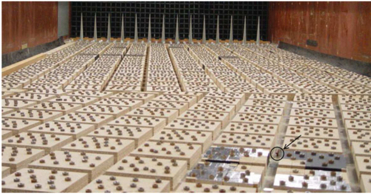
Fig. 1 Wind-tunnel experimental set-up and source position
